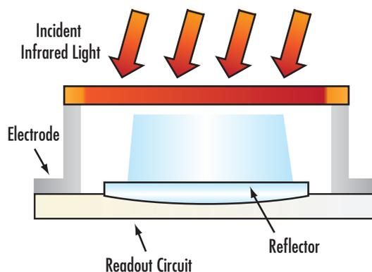
Figure 3: Illustration of Cross-Section of Microbolometer Sensor Array
