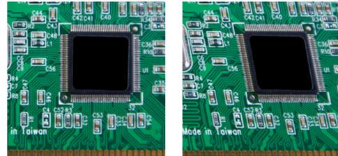
Figure 7b: Comparison of Motion Blur in Global and Rolling Shutters. Sensor Chip on a Slow-Moving Conveyor with Global Shutter (Left) and Rolling Shutter (Right)
