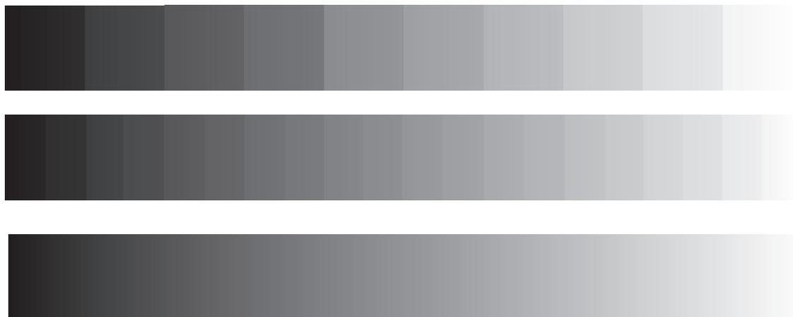
Figure 5: Illustration of 2-Bit (Top), 4-Bit (Middle), and 8-Bit (Bottom) Grayscale
