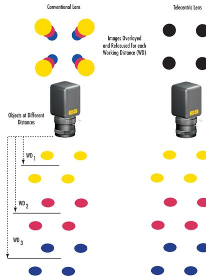
Figure 4: Reduced Perspective Error in Telecentric Lens vs. Conventional Lens
