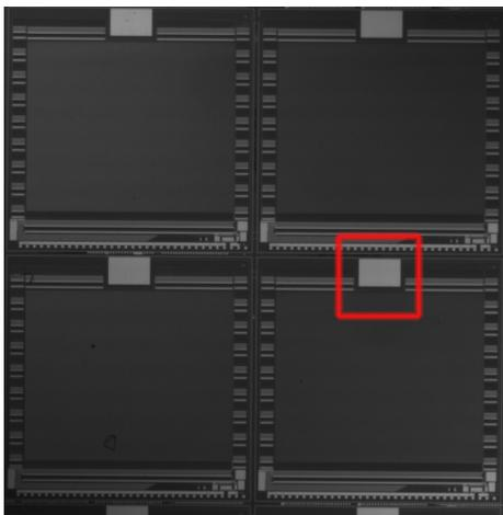
Figure 1a: Real-World Image without Gain (AGC = 0), Gamma = 1, 8MHz Pixel Clock, and 0.2ms Exposure
