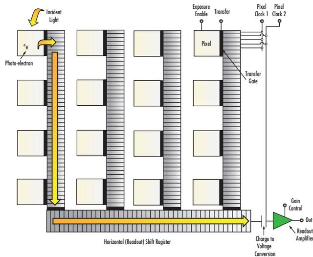
Figure 1: Block Diagram of a Charge-Coupled Device (CCD)
