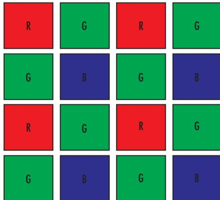
Figure 9a: Single-Chip Color CCD Camera Sensor using Mosaic Filter to Filter Colors
