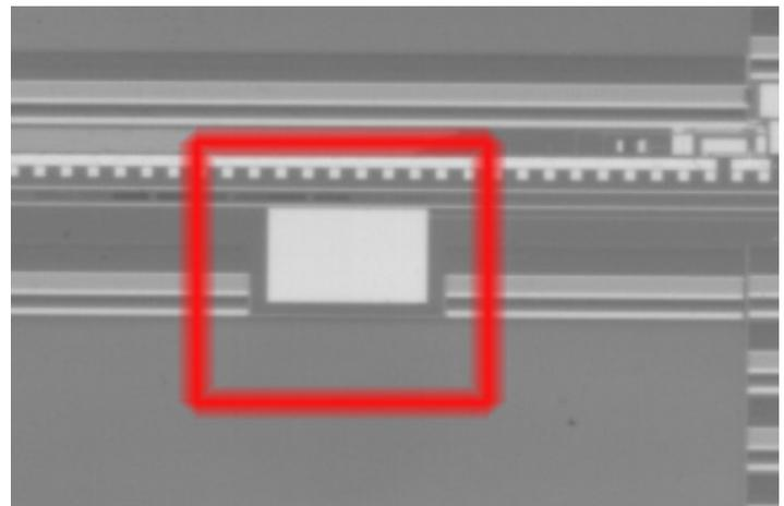
Figure 4b: Close-Up of Image with Gamma = 2, 10MHz Pixel Clock, and 5ms Exposure
