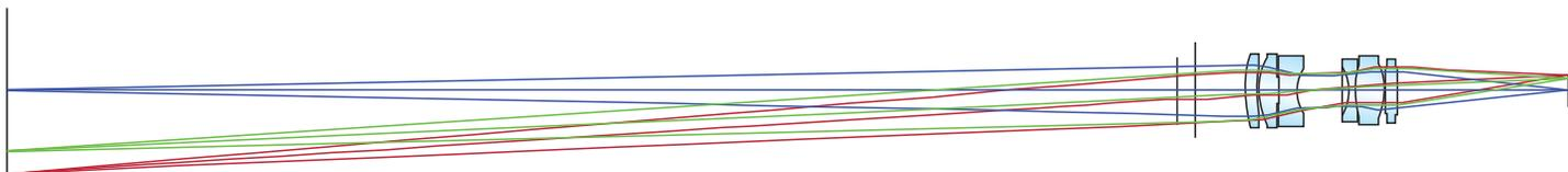
Figure 5: 75mm FL Conventional Lens (Note the Chief Rays in Both Image and Object Spaces are NOT Parallel)
