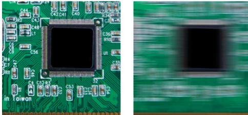
Figure 7a: Comparison of Motion Blur. Sensor Chip on a Fast-Moving Conveyor with Triggered Global Shutter (Left) and Continuous Global Shutter (Right)
