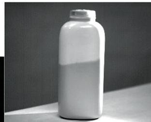
**Figure 3b: SWIR Imaging of Baby Powder Bottle.** The Bottle is Transparent to SWIR Wavelengths. It is Easy to See the Amount of Powder Within.
