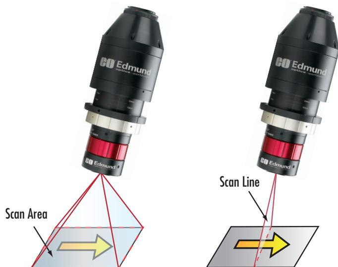
Figure 2: Illustration of Area Scanning Technique (left). Illustration of Line Scanning Technique (right)
