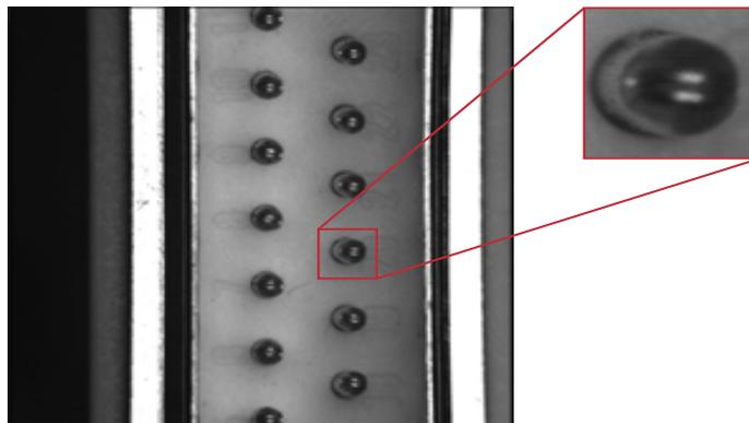
Figure 7: Conventional Lens Imaging Jumper Pins
