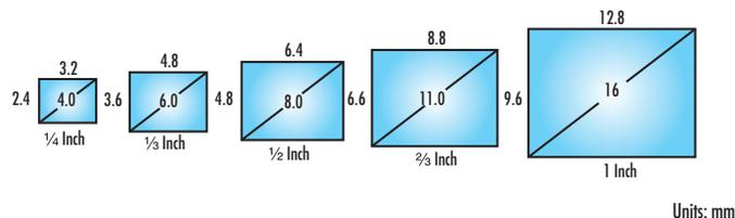
Figure 5: Illustration of Sensor Size Dimensions for Standard Camera Sensors
