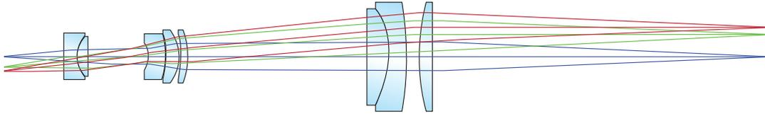
Figure 2: 0.5X Image-Space Telecentric Lens (Note the Parallel Chief Rays in Image Space)
