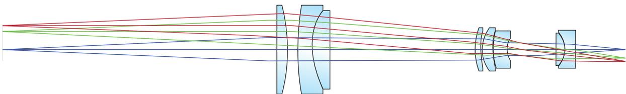
Figure 1: 0.5X Object-Space Telecentric Lens (Note the Parallel Chief Rays in Object Space)
