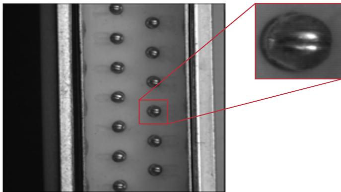
Figure 6: Telecentric Lens Imaging Jumper Pins
