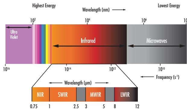
Figure 1: Electromagnetic Spectrum Illustrating SWIR Wavelength Range
