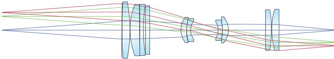
Figure 3: 0.9X Double Telecentric Lens (Note the Parallel Chief Rays in Both Image and Object Spaces)
