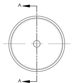
4mm .16in 3mm /1 M3 x 0.5 THRU ONE WALL-.12in 3mm .12in Ø 25mm 2X M23.2 x 0.75 .98in 10mm **SECTION A-A**
