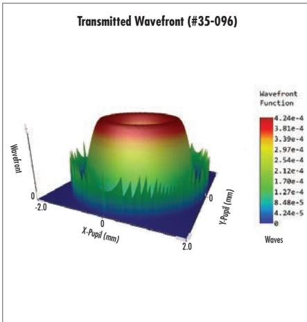
The design wavefront for the 3X 266nm beam expander (#35-096) displayed allows for a  $\lambda/10$  specification for transmitted wavefront.
