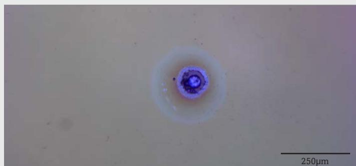
**Figure 1:** Coating failure caused by a UV laser
