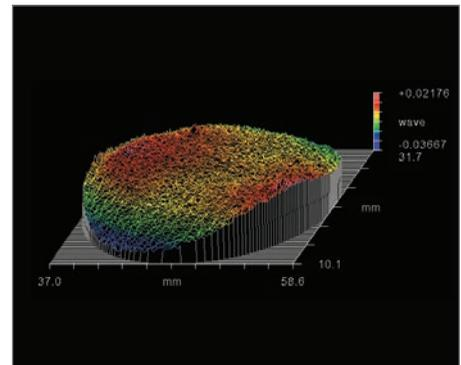
Surface flatness is measured interferometrically. A typical test for #34-820 shows significantly better surface figure after coating than the λ/10 specification.
