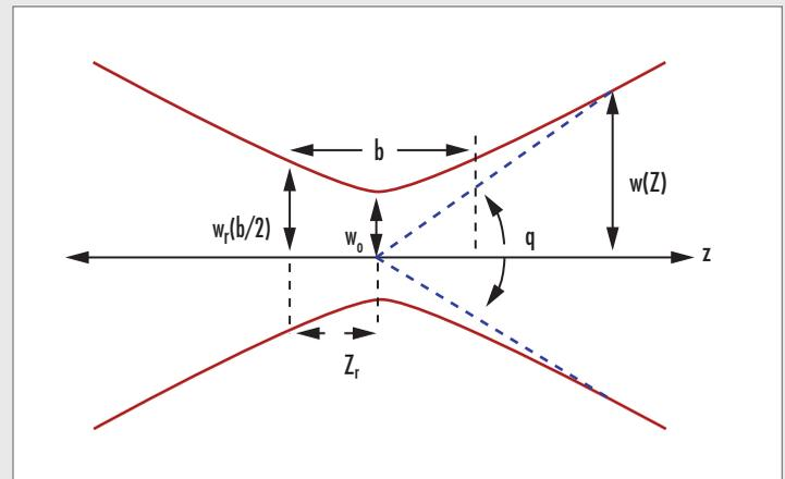
Figure 1: Profile of a Gaussian beam
