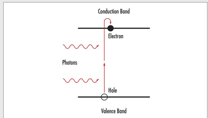
Figure 2: Multiphoton absorption exciting an electron into the conduction band, causing light that would normally be transmitted to be absorbed
