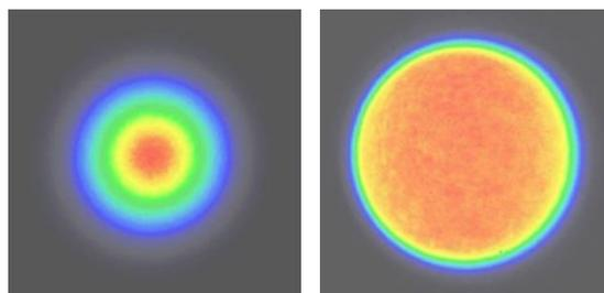
Angular magnification of the telescopic system is about 0.65. Thus, from the point of view of paraxial optics, the diameter of the output beam is increased by factor 1/0.65 while the field angle is reduced by a factor 0.65.
