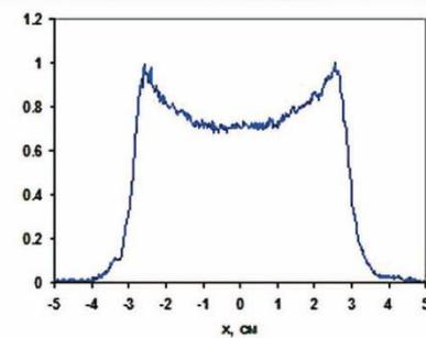
Figure 10. Flat Top Beam Shaper operation by variable diameter of perfect Gaussian input beam.
