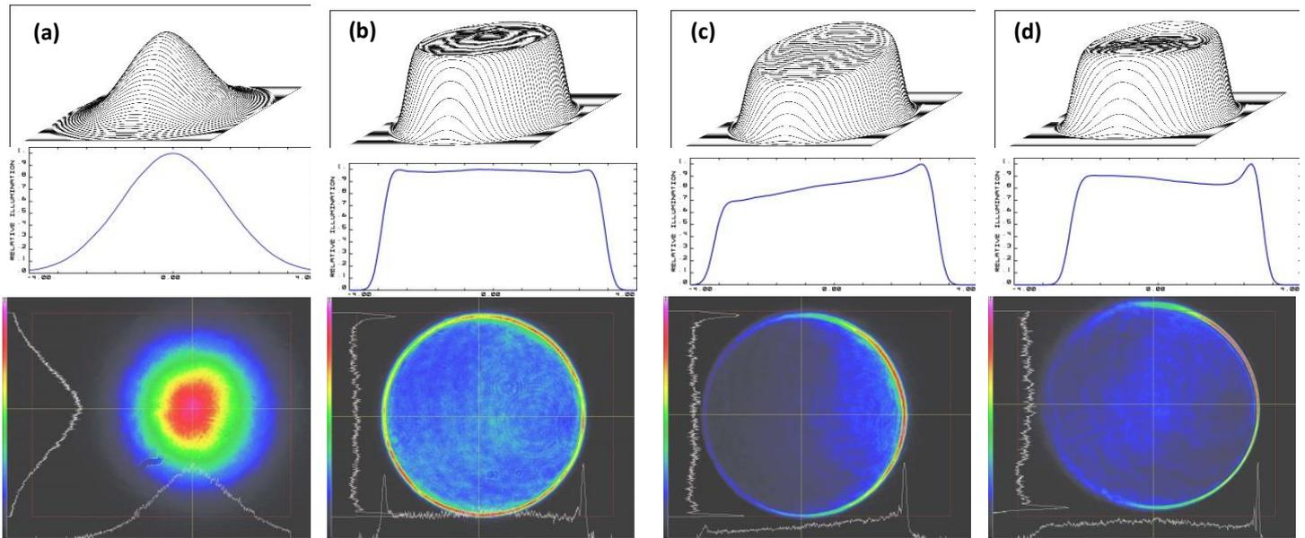
Figure 12 To evaluation of sensitivity of misalignments, theoretical and experimental intensity profiles for Flat Top Beam Shaper 6\_6\_1064 @ 1064nm:
