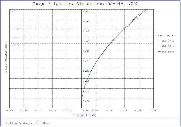
#55-349, 0.25X 2/3" GoldTL™ Telecentric Lens, Distortion Plot
