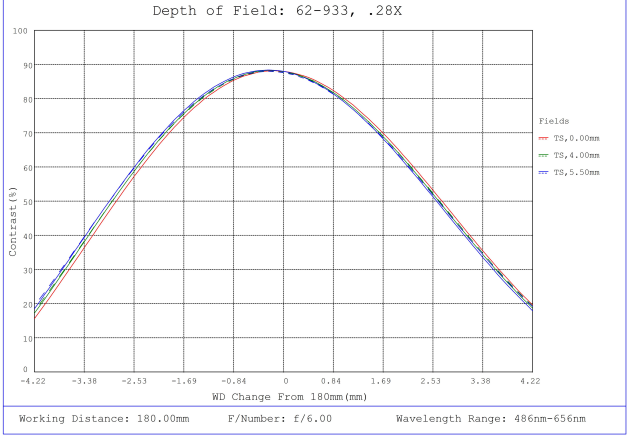
#62-933, 0.28X, 2/3" C-Mount PlatinumTL™ Telecentric Lens, Depth of Field Plot, 180mm Working Distance, f6
