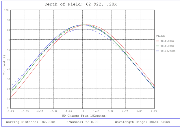
#62-922, 0.28X, 28.7mm F-Mount PlatinumTL™ Telecentric Lens, Depth of Field Plot, 182mm Working Distance, f10
