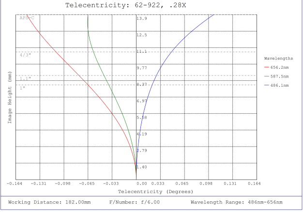
#62-922, 0.28X, 28.7mm F-Mount PlatinumTL™ Telecentric Lens, Telecentricity Plot
