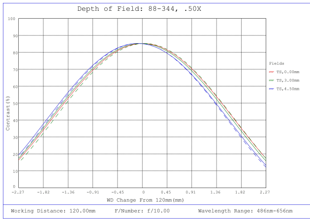
#88-344, 0.50X In-Line Illumination SilverTL™ Telecentric Lens, Depth of Field Plot, 120mm Working Distance, f10
