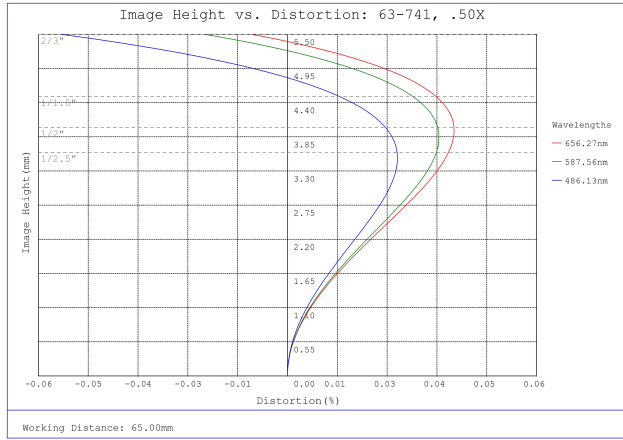
#63-741, 0.5X, 65mm WD CompactTL™ Telecentric Lens, Distortion Plot
