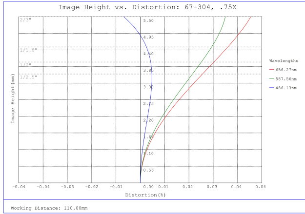
#67-304, 0.75X, 110mm WD, In-Line CompactTL™ Telecentric Lens, Distortion Plot
