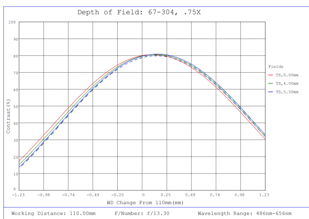
#67-304, 0.75X, 110mm WD, In-Line CompactTL™ Telecentric Lens, Modulated Transfer Function (MTF) Plot, 110mm Working Distance, f13.3
