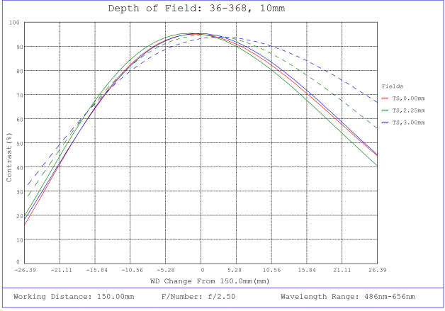
#36-368, 10mm FL f/2.5, Rugged Blue Series M12 Lens, Depth of Field Plot, 150mm Working Distance, f2.5
