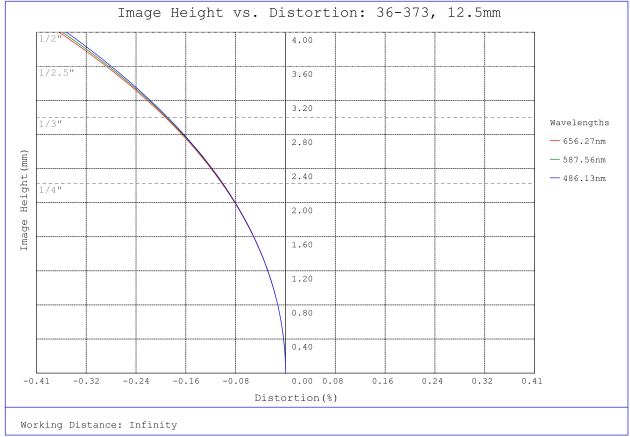
#36-373, 12.5mm FL f/4, Rugged Blue Series M12 Lens, Distortion Plot
