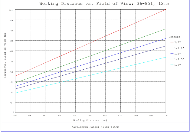
#36-851, 12mm f/2.8, 1000mm-∞ Primary WD, HRr Series Fixed Focal Length Lens, Working Distance versus Field of View Plot
