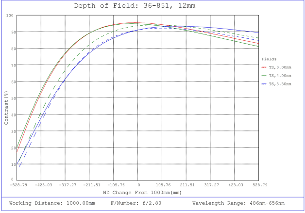
#36-851, 12mm f/2.8, 1000mm-∞ Primary WD, HRr Series Fixed Focal Length Lens, Depth of Field Plot, 1000mm Working Distance, f2.8
