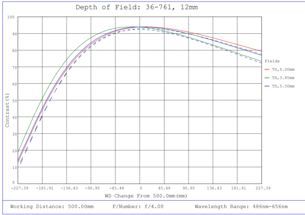
#36-761, 12mm f/4, 400-2000mm Primary WD, HRI Series Fixed Focal Length Lens, Depth of Field Plot, 500mm Working Distance, f4
