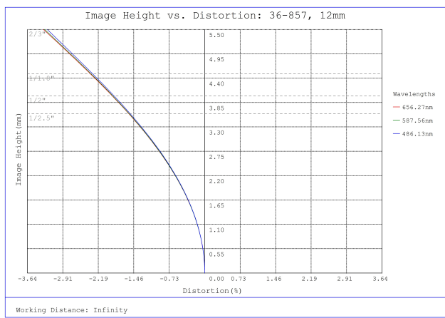
#36-857, 12mm f/5.6, 1000mm-∞ Primary WD, HRr Series Fixed Focal Length Lens, Distortion Plot
