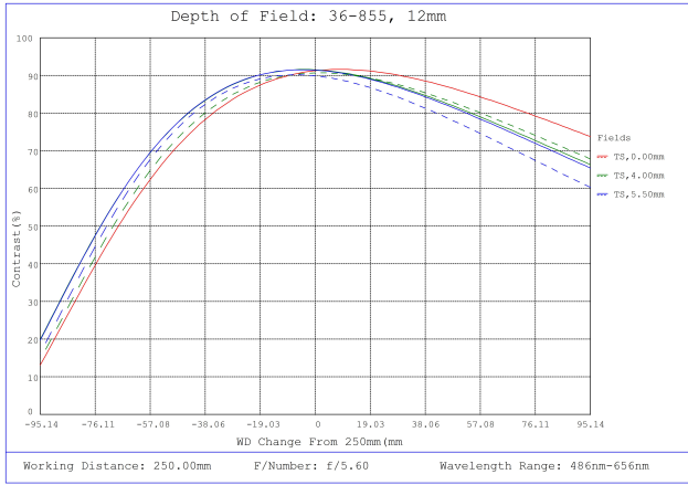
#36-855, 12mm f/5.6, 150-500mm Primary WD, HRr Series Fixed Focal Length Lens, Depth of Field Plot, 250mm Working Distance, f5.6
