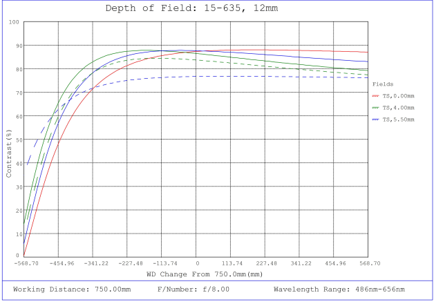
#15-635, 12mm, f/8 Cw Series Fixed Focal Length Lens, Depth of Field Plot, 750mm Working Distance, f8
