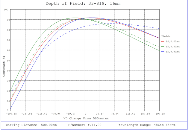
#33-819, 16mm f/11, HPi Series Fixed Focal Length Lens, Depth of Field Plot, 500mm Working Distance, f11
