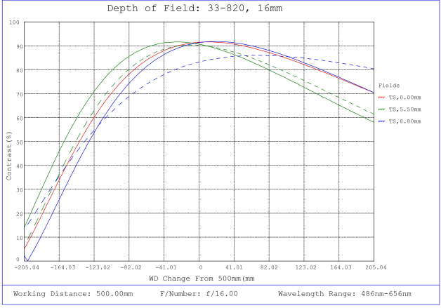
#33-820, 16mm f/16, HPi Series Fixed Focal Length Lens, Depth of Field Plot, 500mm Working Distance, f16
