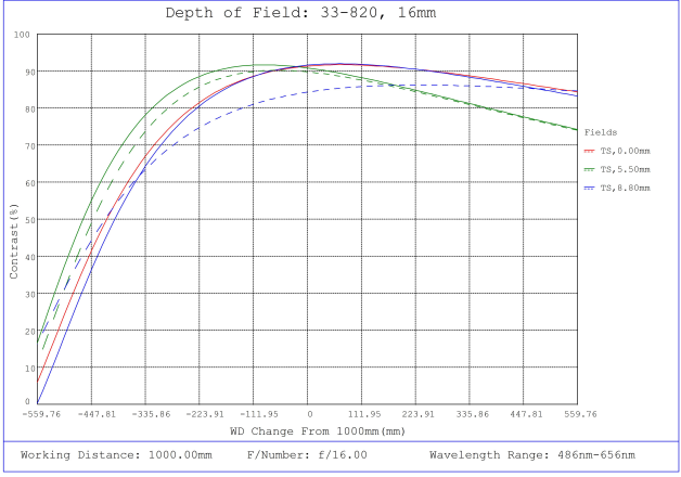
#33-820, 16mm f/16, HPi Series Fixed Focal Length Lens, Depth of Field Plot, 1000mm Working Distance, f16
