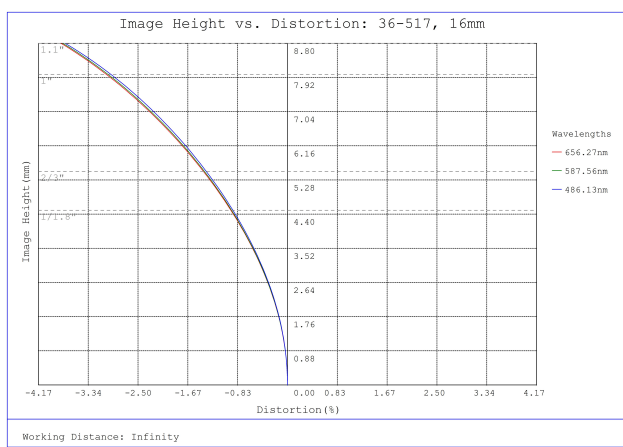
#36-517, 16mm f/16, HPr Series Fixed Focal Length Lens, Distortion Plot
