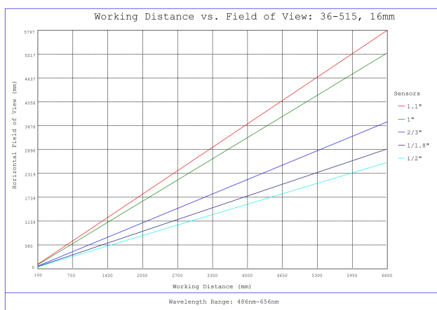
#36-515, 16mm f/8, HPr Series Fixed Focal Length Lens, Working Distance versus Field of View Plot
