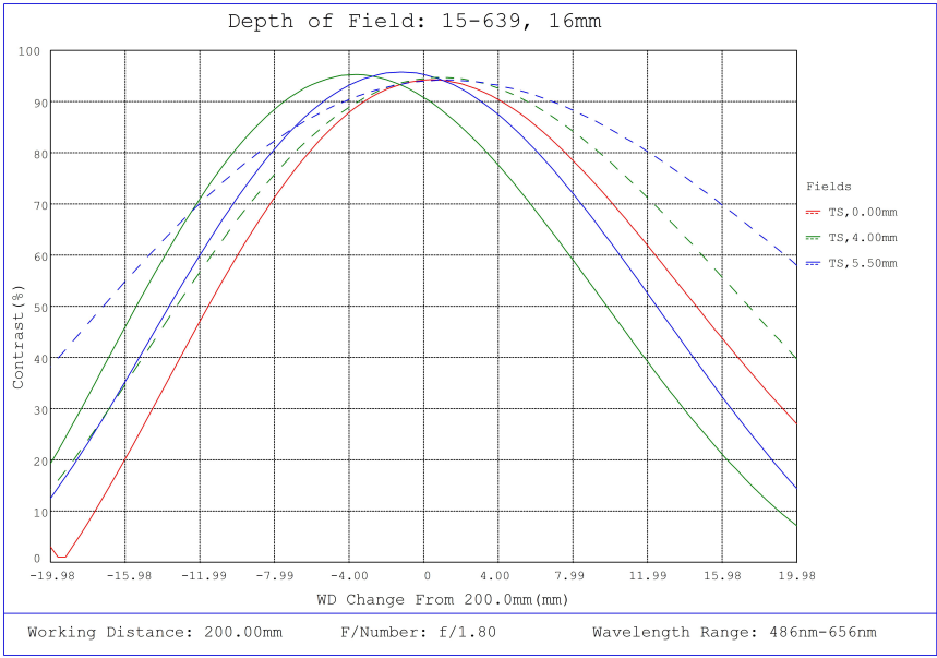
#15-639, 16mm, f/1.8 Cw Series Fixed Focal Length Lens, Depth of Field Plot, 200mm Working Distance, f1.8
