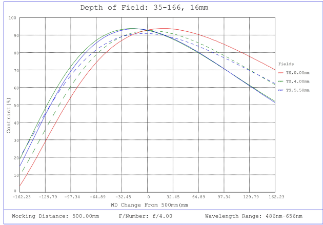
#35-166, 16mm, f/4 Cr Series Fixed Focal Length Lens, Depth of Field Plot, 500mm Working Distance, f4
