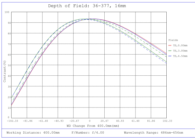
#36-377, 16mm FL f/4.0 Rugged Blue Series M12 Lens, Depth of Field Plot, 400mm Working Distance, f4
