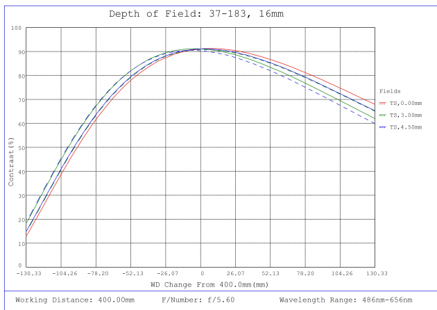
#37-183, 16mm FL f/5.6 Blue Series M12 Lens, Depth of Field Plot, 400mm Working Distance, f5.6
