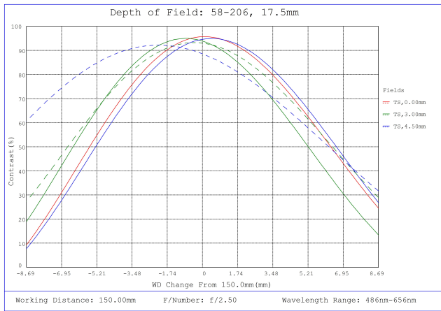
#58-206, 17.5mm FL f/2.5, Blue Series M12 Lens, Depth of Field Plot, 150mm Working Distance, f2.5
