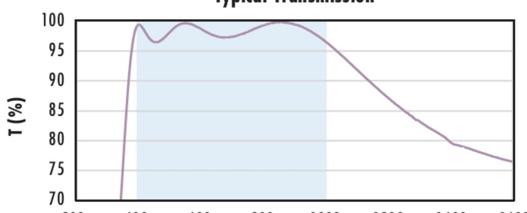
Typical transmission of a 3mm thick N-BK7 window with MS-NIR (400-1000nm) coating at 0° AOI.
