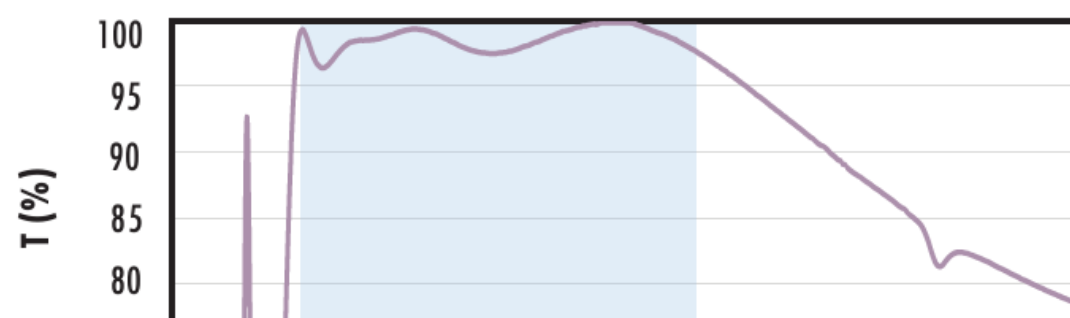
Fused Silica with VIS-NIR Coating Typical Transmission
