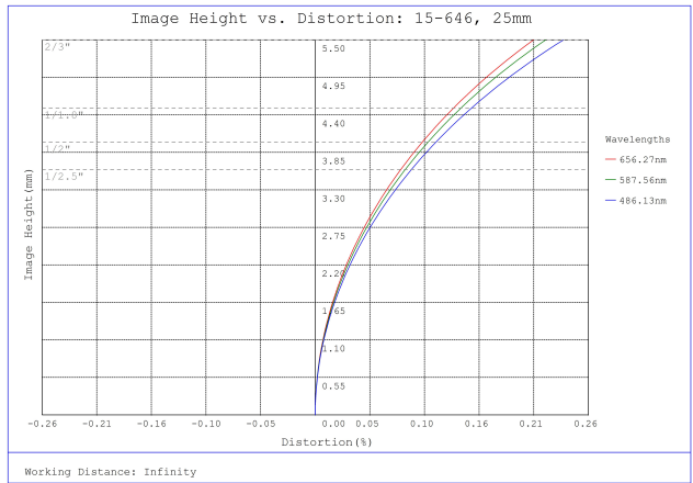
#15-646, 25mm, f/1.6 Cw Series Fixed Focal Length Lens, Distortion Plot
