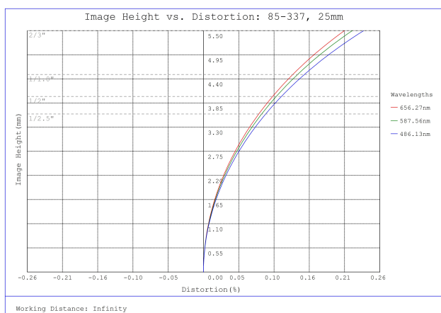
#85-337, 25mm, f/16 Ci Series Fixed Focal Length Lens, Distortion Plot
