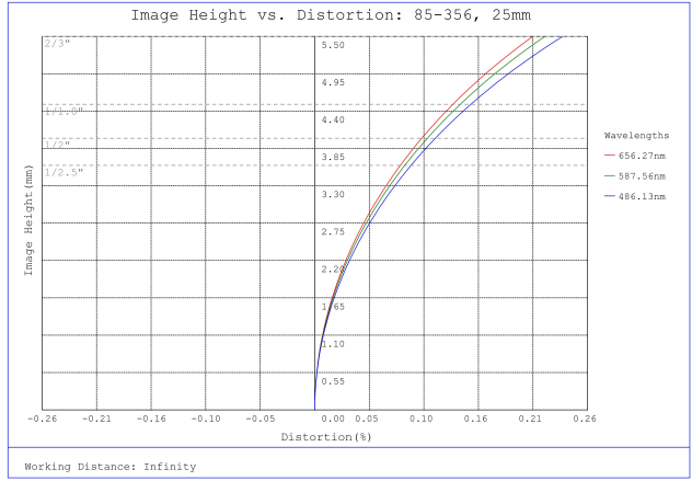
#85-356, 25mm, f/1.8 Ci Series Fixed Focal Length Lens, Distortion Plot
