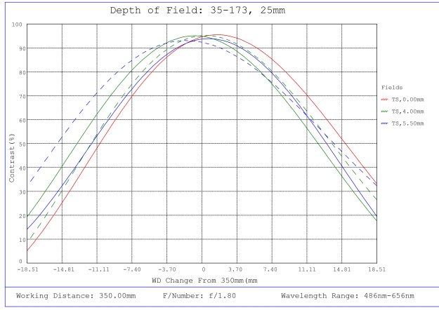
#35-173, 25mm, f/1.8 Cr Series Fixed Focal Length Lens, Depth of Field Plot, 350mm Working Distance, f1.8
