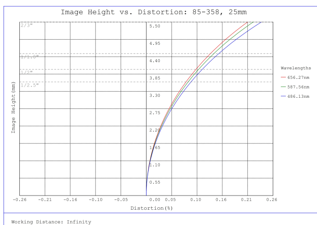
#85-358, 25mm, f/4 Ci Series Fixed Focal Length Lens, Distortion Plot
