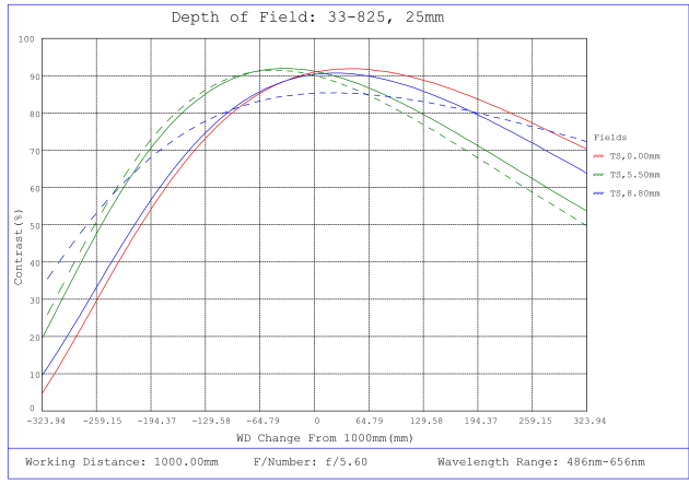
#33-825, 25mm f/5.6, HPi Series Fixed Focal Length Lens, Depth of Field Plot, 1000mm Working Distance, f5.6
