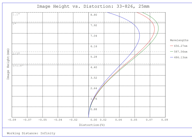
#33-826, 25mm f/8.0, HPI Series Fixed Focal Length Lens, Distortion Plot
