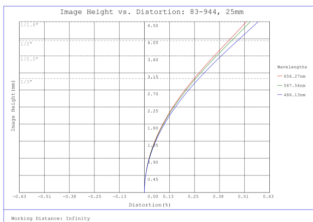
#83-944, 25mm FL f/5.6, Blue Series M12 Lens, Distortion Plot
