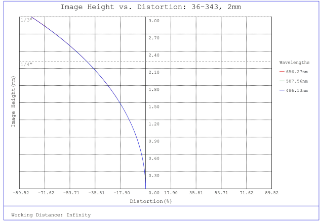
#36-343, 2mm FL f/2.5 Rugged Blue Series M12 Lens, Distortion Plot
