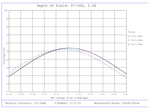
#67-306, 2X, 110mm WD, In-Line CompactTL™ Telecentric Lens, Depth of Field Plot, 110mm Working Distance, f33
