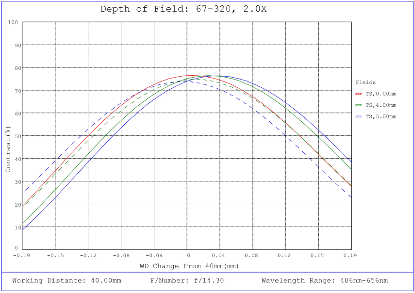
#67-320, 2X, 40mm WD, In-Line CompactTL™ Telecentric Lens, Depth of Field Plot, 40mm Working Distance, f14.3
