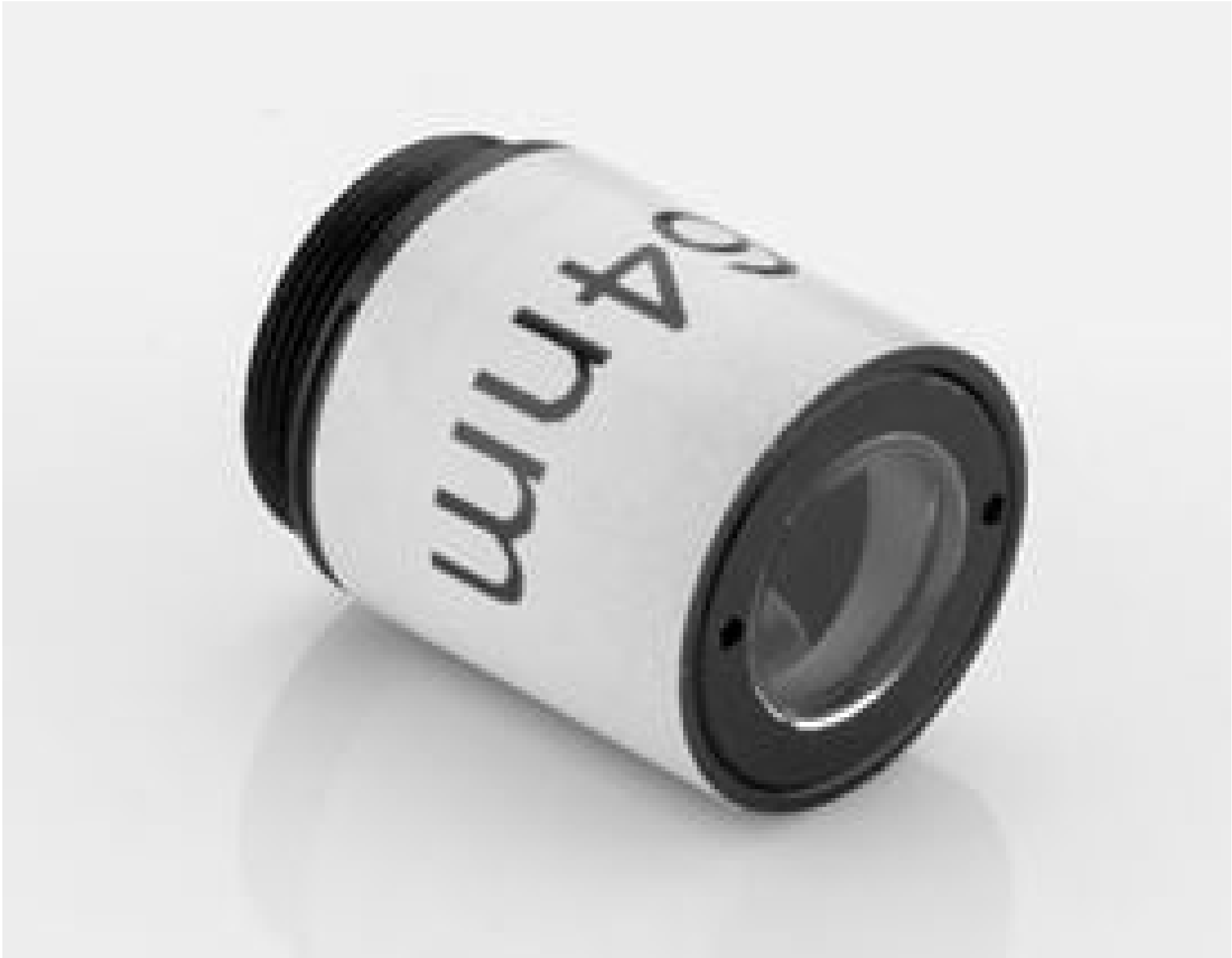
#37-097: 30°, 1064nm Single Line Projection Head
