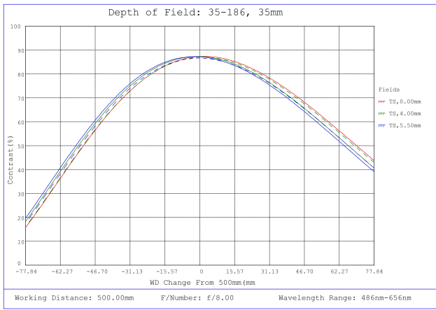
#35-186, 35mm, f/8.0 Cr Series Fixed Focal Length Lens, Depth of Field Plot, 500mm Working Distance, f8
