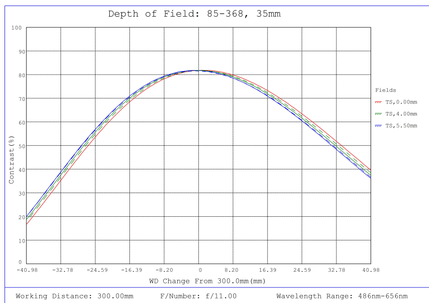
#85-368, 35mm, f/11 Ci Series Fixed Focal Length Lens, Depth of Field Plot, 300mm Working Distance, f11
