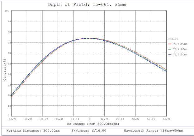
#15-661, 35mm, f/16 Cw Series Fixed Focal Length Lens, Depth of Field Plot, 300mm Working Distance, f16
