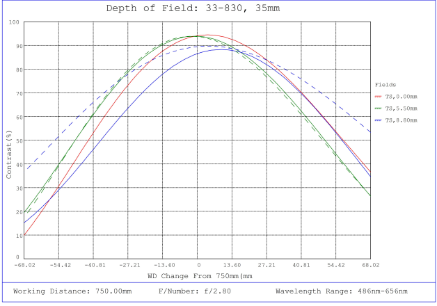
#33-830, 35mm f/2.8, HPi Series Fixed Focal Length Lens, Depth of Field Plot, 750mm Working Distance, f2.8
