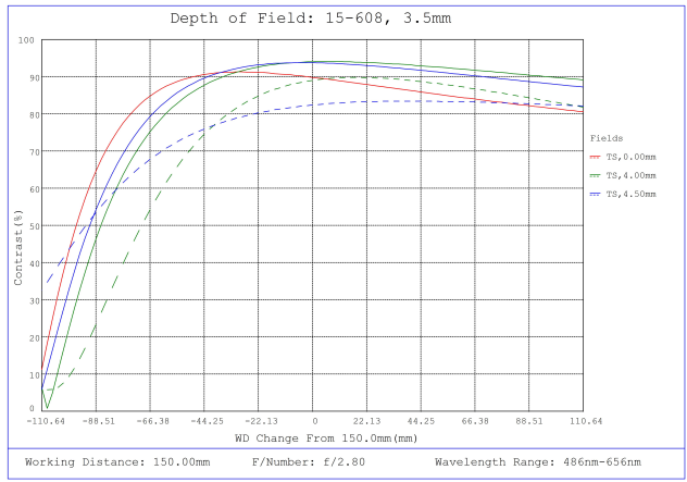
#15-608, 3.5mm f/2.8 Sealed Cw Series Fixed Focal Length Lens, Depth of Field Plot, 150mm Working Distance, f2.8
