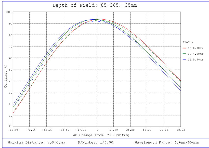
#85-365, 35mm, f/4 Ci Series Fixed Focal Length Lens, Depth of Field Plot, 750mm Working Distance, f4
