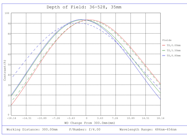
#36-528, 35mm f/4.0, HPr Series Fixed Focal Length Lens, Depth of Field Plot, 300mm Working Distance, f4
