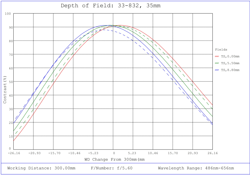
#33-832, 35mm f/5.6, HPI Series Fixed Focal Length Lens, Depth of Field Plot, 300mm Working Distance, f5.6
